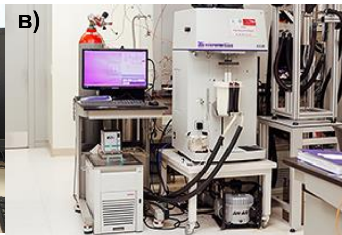
c) System for determination of specific surface area and size of pores
